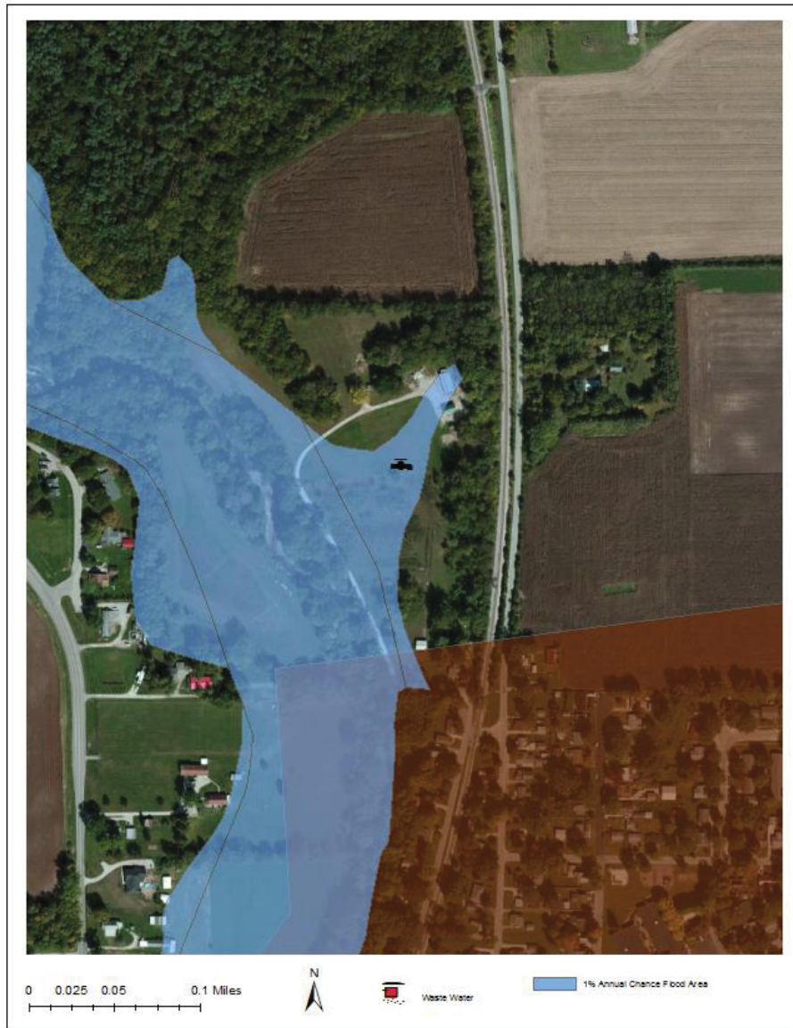
Figure 16: Boundary of 1% Annual Chance Flood Overlaid within Tippecanoe County Unincorporated area Critical Facilities
